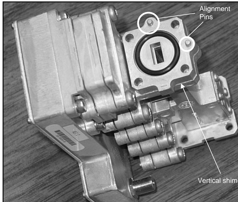
Figure 5. Vertical shim installed on TRIA
